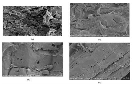
Gambar 1. (a) kulit durian murni, 10.9mm × 1.00k SE; (b) HAMDP, 11.2mm × 3.0k SE; (c) biosorben setelah adsorpsi Zn (II), 11.2mm × 3.00k SE dan (d) biosorben setelah Zn (II) desorpsi, 11.3mm × 1.00k SE. (Ngabura et al.,2018)
